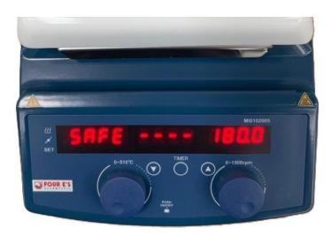
The hotplate stirrer has a safety (maximum) temperature setting. This is adjusted using the supplied screwdriver through the hole next to the power on/off switch. Once you start to adjust the setting (turning the screw), the display will show the word SAFE and the current safety setting.
