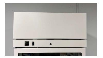
With the controller cover now in place, you can reinstall the front panel. Place the panel slightly above it's final position matching the rectangular holes with the locating blocks.
