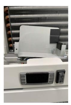
Reattach the wires of the various sensors to the controller using the supplied wiring schematic on the next page. Once the wires are connected, slide the reattached controller back through the front panel
