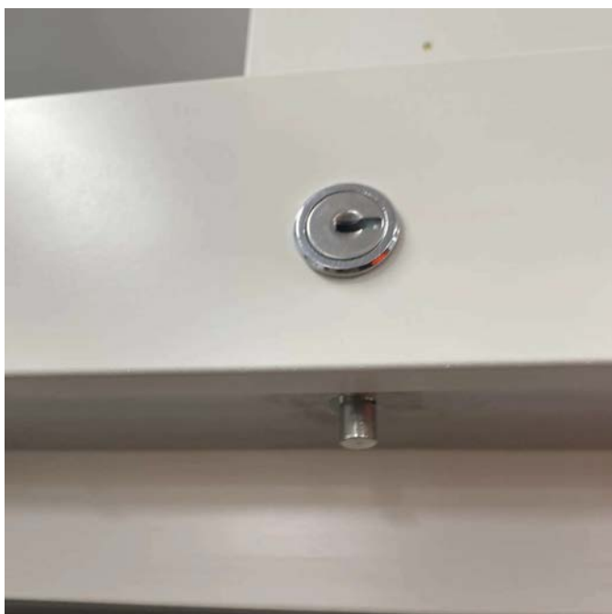
Unscrew the locking pin under the lock and remove it using long nose pliers.
