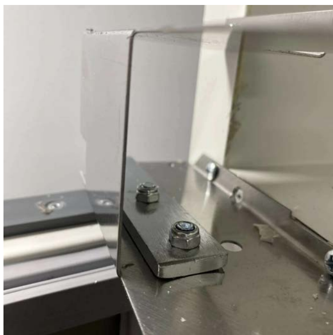
To access the screws that hold the top hinge pin bracket in place, the door needs to be opened to a 90° angle.
