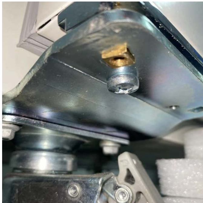
The square end will still sit in the plate but will allow the door to be lifted once the top hinge pin bracket is released.
