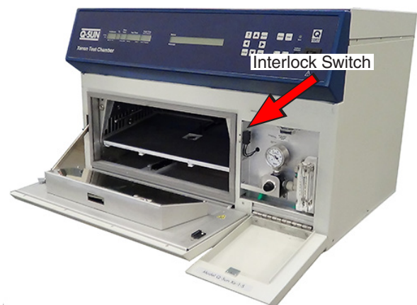
Figure 2f: Basic model tester chamber door interlock switch location (test chamber and plumbing access door open).
