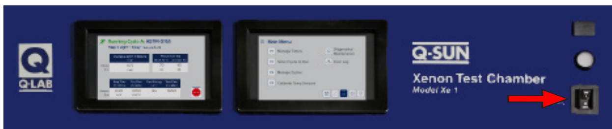
Figure 7.2a: Power switch on Xe-1-SE, Xe-1-BCE, Xe-1-SCE, and Xe-1-WE control panel.
