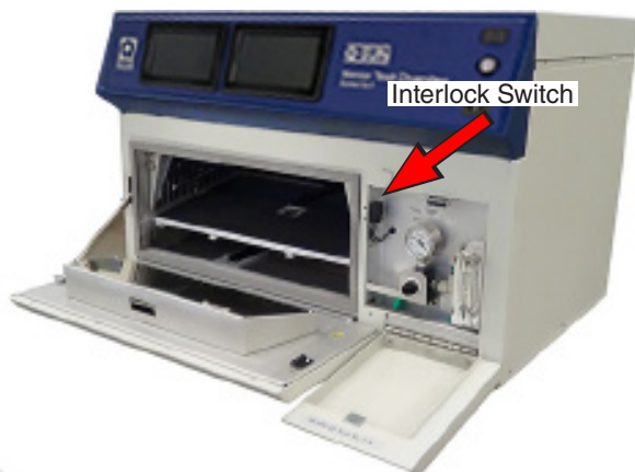
Figure 2e: "E" model testers chamber door interlock switch location (test chamber and plumbing access door open).
