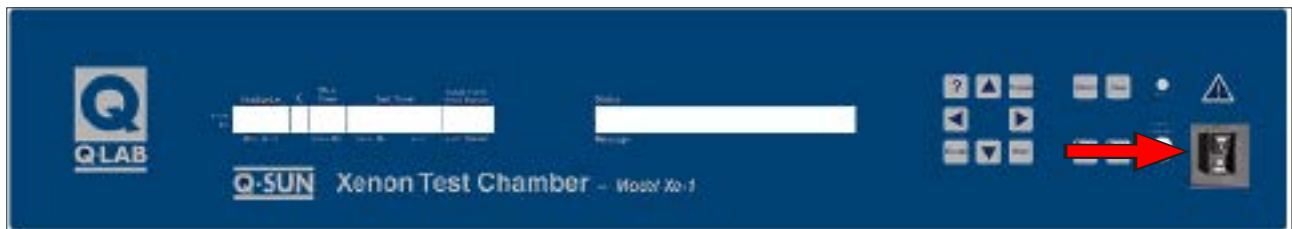
Figure 7.3a: Power switch on Xe-1-B control panel.
