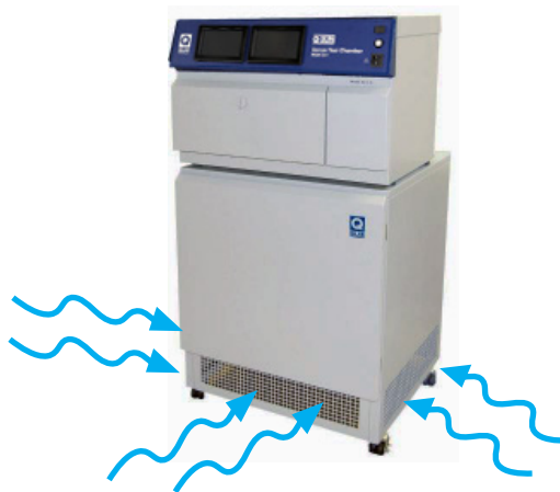
Figure 6.4c: Q-SUN Xe-1-BCE and Xe-1-SCE chiller cooling air intake areas.
