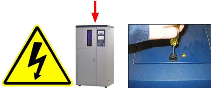
Figure 2.1c: Lamp door located on top of the Xe-2 cabinet.
