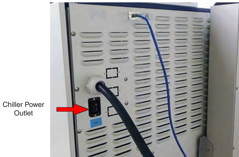
Figure 5.8h: Power outlet for chiller on Xe-3 rear panel.
