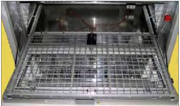
Figure 6.5b: Open mesh specimen tray - install under horizontal specimen tray insert.
