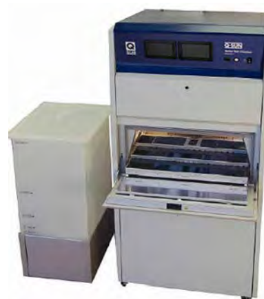
Figure 5.6h: Position the Dual Spray assembly next to Xe-3 as shown.
