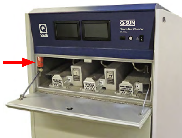
Figure 2.1d: Lamp Door Interlock Switch Location
