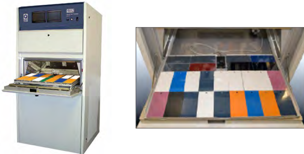
Figure 6.1: Xe-3 Specimen tray pulled out and specimens placed on tray.
