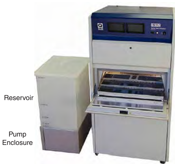
Figure 2.3: Dual Spray reservoir and pump system enclosure.
