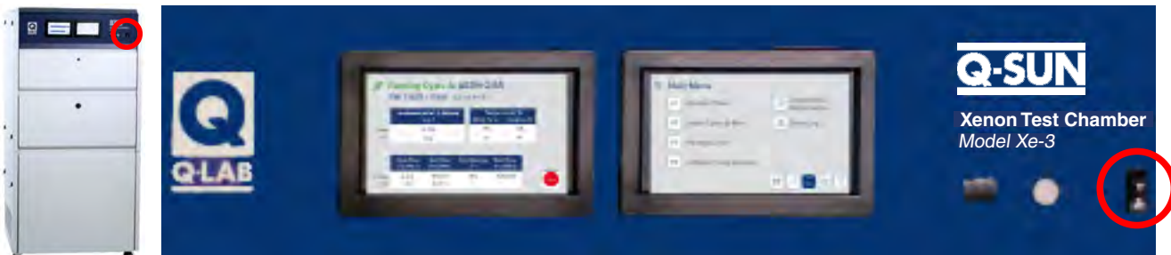
Figure 6.2a: Power switch on control panel of all “E” model Xe-3 testers.
