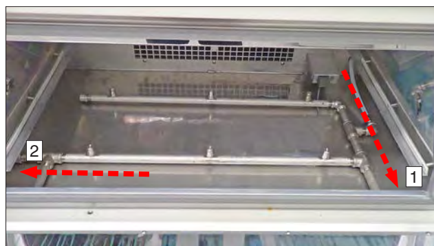
Figure 5.5b: Remove tape. Slide the manifold forward, then to the left.
