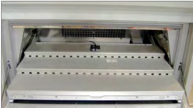
Figure 6.5a: Horizontal specimen tray insert - install on open mesh tray so liquid will not run off the specimens.
