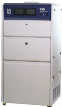
Figure 4.2a: Do not install testers in a room with corrosion chambers.
