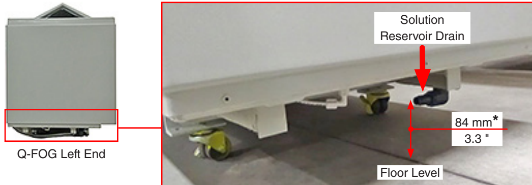
Figure 5.8d: Solution reservoir drain location with 70 mm (2.75") high optional caster.
