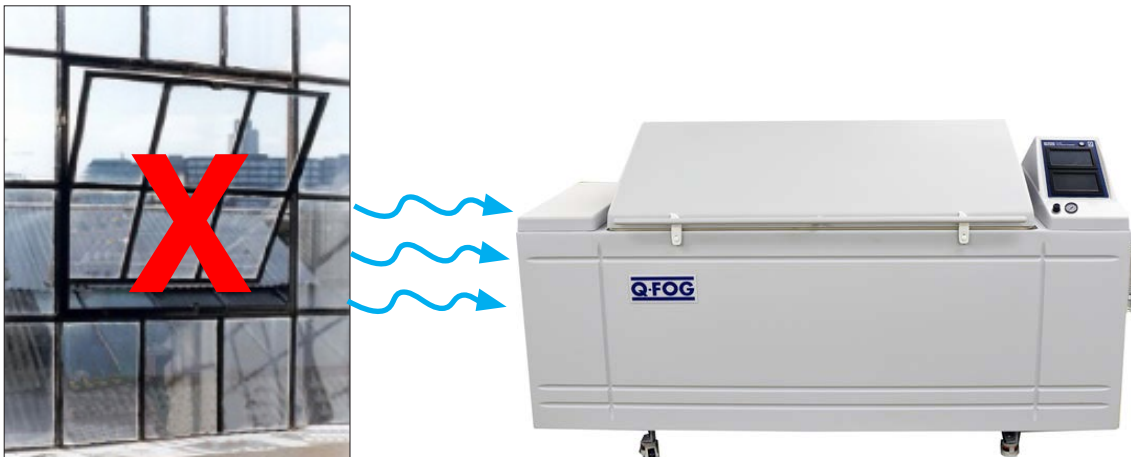
Figure 4.2c: Do not locate Q-FOG near open windows.
