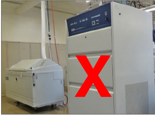
Figure 4.2a: Do not install Q-FOG in a room with Q-SUN or QUV testers.
