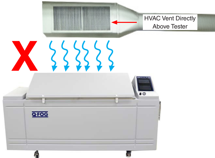
Figure 4.2d: Keep tester away from sources of hot or cold air.
