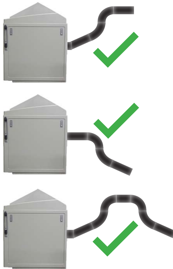
Figure 5.9f: Correct vent installations.
