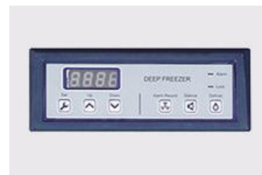
Microprocessor control panel
