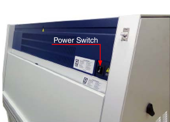
Figure 7.2a: Power switch located on rear of tester.
