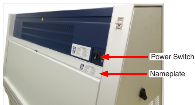
Figure 6.3: QUV rear view showing power switch and nameplate and locations.
