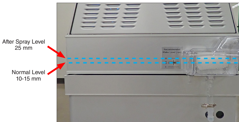
Figure 6.4i: Normal and after-spray water levels.
