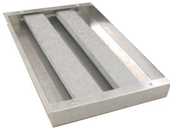
Figure 7.1f: Wide 3D specimen holder with clamps.
