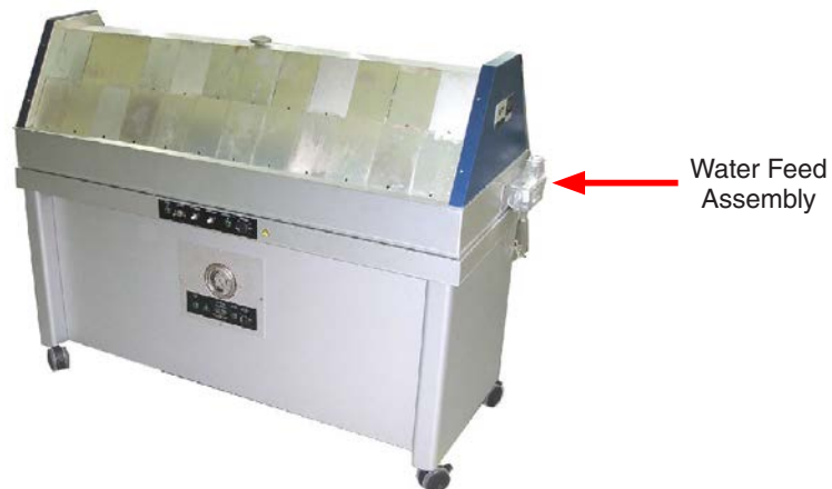
Figure 6.4b: QCT water supply connection location.
