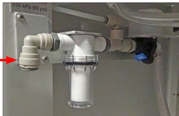
Figure 6.4f: Push lock elbow for ½" water supply tube
